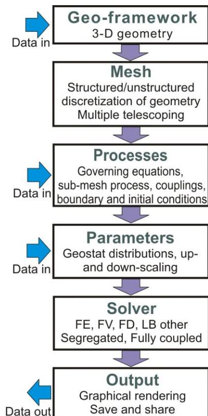
Figure 1. Major modules and basic workflow for developing an analysis using the Community Water Model.
